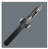
Four screw sizes can be operated with the 4-in-1 bits 9506 and 9507. The 4-in-1 bit 9506 for four sizes of hexagonal socket screws (3.0; 4.0; 5.0; 6.0), the 4-in-1 bit 9507 for three sizes of hexagonal socket screws (2.5; 5.0; 6.0) and one size of TORX® screws (TX 25). In order to use the larger profile, continuously press against the spring tension while screwdriving so that the smaller profile is countersunk and the larger profile can be used.
